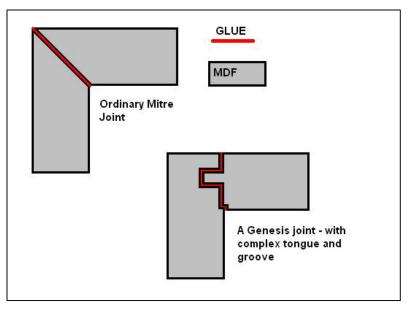
Genesis designed a unique tongue and groove joint in order to improve the structural rigidity of the cabinet.
